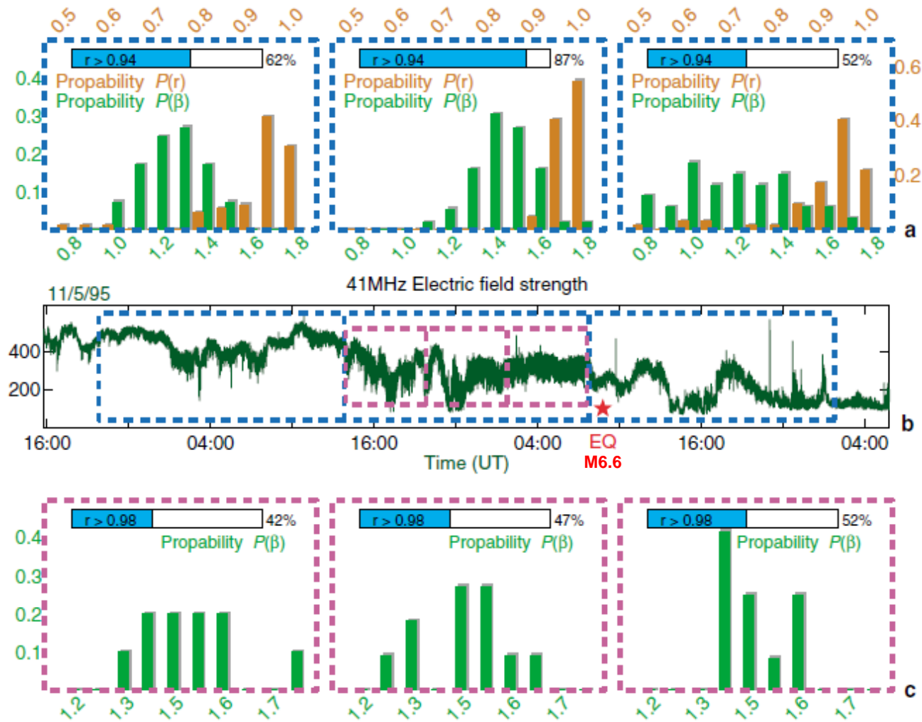
(a) Histograms of probability distribution of the correlation coefficient r and exponent calculated on 1024 measurements segments for three consecutive time intervals (blue frames) marked in (b). Insets show the percentage of segments with r > 0.94 . (b) The time series of the 41 MHz field strength [4]. The star indicates the time of the earthquake occurrence. (c) The probability distribution of the exponent and the percentage of segments with r > 0.98 for 3 consecutive subintervals (purple frames) of 6 h duration each as marked in (b).
